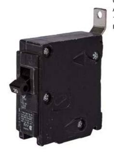
Siemens Low Voltage Molded Case Circuit Breakers Panelboard Mounting 240V Circuit Breakers - Type BL, 1-Pole, 120VAC are Circuit Protection Molded Case Circuit Breakers. Type: BL Application: Electrical Distribution Standard: UL 489 Voltage Rating: 120V Amperage Rating: 60A Trip Range: Thermal Magnetic Interrupt Rating: 10 AIC Number Of Poles: 1P
