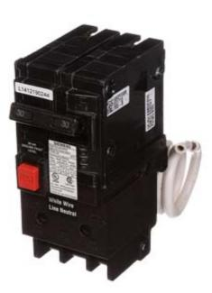
Siemens Low Voltage Residential Circuit Breakers Miniature Circuit Breakers GFCI - Equipment Protect 2-pole plug-on 10k are Circuit Protection Load Center Mains, Feeders, and Miniature Circuit Breakers. Sub Brand: N/A Type: QE Special Features: N/A Application: Electrical Distribution Standard: UL 489 Voltage Rating: 120/240 V Amperage Rating: 30A Load Rating: N/A Frequency Rating: N/A Phase: N/A Frame: N/A Trip Type: N/A Trip Range: Thermal Magnetic Interrupt Rating: 10 AIC Number Of Poles: 2P
