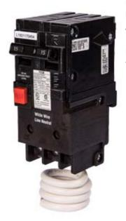
Siemens Low Voltage Residential Circuit Breakers Miniature Circuit Breakers GFCI - Equipment Protect 2-pole plug-on 10k are Circuit Protection Load Center Mains, Feeders, and Miniature Circuit Breakers. Sub Brand: N/A Type: QE Special Features: N/A Application: Electrical Distribution Standard: UL 489 Voltage Rating: 120/240 V Amperage Rating: 15A Load Rating: N/A Frequency Rating: N/A Phase: N/A Frame: N/A Trip Type: N/A Trip Range: Thermal Magnetic Interrupt Rating: 10 AIC Number Of Poles: 2P
