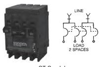
QT Quadplex These space saver quadplex breakers provide two sets of common trip, two-pole breakers for 120/240V AC circuits, and require two panel spaces. HACR rated. J
