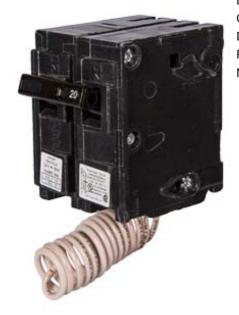
Siemens Low Voltage Residential Circuit Breakers Miniature Thermal Mag Circuit Breakers - Type QP/MP 1-pole 10k are Circuit Protection Load Center Mains, Feeders, and Miniature Circuit Breakers. Type: QP/MP Special Features: Shunt Trip 120V Application: Electrical Distribution Standard: UL 489 Voltage Rating: 120V Amperage Rating: 30A Trip Range: Thermal Magnetic Interrupt Rating: 10 AIC Number Of Poles: 1P
