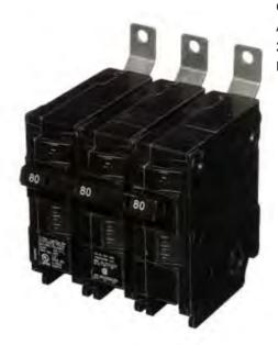
Siemens Low Voltage Molded Case Circuit Breakers Panelboard Mounting 240V Circuit Breakers - Type BL, 3-Pole, 240VAC are Circuit Protection Molded Case Circuit Breakers. Type: BL Application: Electrical Distribution Standard: UL 489 Voltage Rating: 240V Amperage Rating: 80A Trip Range: Thermal Magnetic Interrupt Rating: 10 AIC Number Of Poles: 3P
