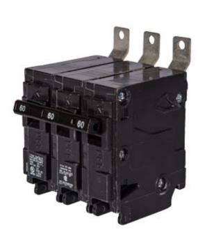
Siemens Low Voltage Molded Case Circuit Breakers Panelboard Mounting 240V Circuit Breakers - Type BL, 3-Pole, 240VAC are Circuit Protection Molded Case Circuit Breakers. Type: HBL Application: Electrical Distribution Standard: UL 489 Voltage Rating: 240V Amperage Rating: 60A Trip Range: Thermal Magnetic Interrupt Rating: 65 AIC Number Of Poles: 3P
