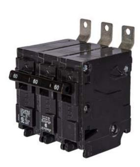
Siemens Low Voltage Molded Case Circuit Breakers Panelboard Mounting 240V Circuit Breakers - Type BL, 3-Pole, 240VAC are Circuit Protection Molded Case Circuit Breakers. Type: BL Application: Electrical Distribution Standard: UL 489 Voltage Rating: 240V Amperage Rating: 60A Trip Range: Thermal Magnetic Interrupt Rating: 10 AIC Number Of Poles: 3P
