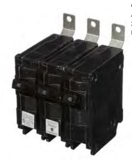
Siemens Low Voltage Molded Case Circuit Breakers Panelboard Mounting 240V Circuit Breakers - Type BL, 3-Pole, 240VAC are Circuit Protection Molded Case Circuit Breakers. Type: BL Application: Electrical Distribution Standard: UL 489 Voltage Rating: 240V Amperage Rating: 45A Trip Range: Thermal Magnetic Interrupt Rating: 10 AIC Number Of Poles: 3P
