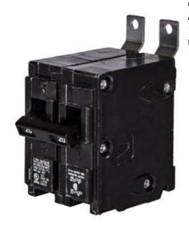
Siemens Low Voltage Molded Case Circuit Breakers Panelboard Mounting 240V Circuit Breakers - Type BL, 2-Pole, 120/240VAC are Circuit Protection Molded Case Circuit Breakers. Type: BLH Application: Electrical Distribution Standard: UL 489 Voltage Rating: 120/240V Amperage Rating: 80A Trip Range: Thermal Magnetic Interrupt Rating: 22 AIC Number Of Poles: 2P
