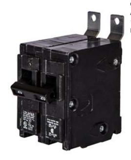
Siemens Low Voltage Molded Case Circuit Breakers Panelboard Mounting 240V Circuit Breakers - Type BL, 2-Pole, 120/240VAC are Circuit Protection Molded Case Circuit Breakers. Type: BLH Application: Electrical Distribution Standard: UL 489 Voltage Rating: 120/240V Amperage Rating: 40A Trip Range: Thermal Magnetic Interrupt Rating: 22 AIC Number Of Poles: 2P
