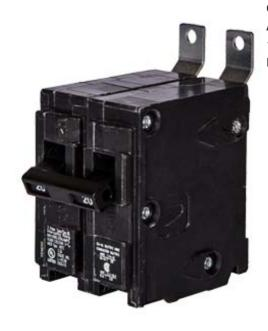
Siemens Low Voltage Molded Case Circuit Breakers Panelboard Mounting 240V Circuit Breakers - Type BL, 2-Pole, 120/240VAC are Circuit Protection Molded Case Circuit Breakers. Type: HBL Application: Electrical Distribution Standard: UL 489 Voltage Rating: 120/240V Amperage Rating: 25A Trip Range: Thermal Magnetic Interrupt Rating: 65 AIC Number Of Poles: 2P
