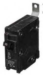
Siemens Low Voltage Molded Case Circuit Breakers Panelboard Mounting 240V Circuit Breakers - Type BL, 1-Pole, 120VAC are Circuit Protection Molded Case Circuit Breakers. Type: BL Application: Electrical Distribution Standard: UL 489 Voltage Rating: 120V Amperage Rating: 30A Trip Range: Thermal Magnetic Interrupt Rating: 10 AIC Number Of Poles: 1P
