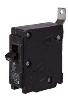
Siemens Low Voltage Molded Case Circuit Breakers Panelboard Mounting 240V Circuit Breakers - Type BL, 1-Pole, 120VAC are Circuit Protection Molded Case Circuit Breakers. Type: HBL Application: Electrical Distribution Standard: UL 489 Voltage Rating: 120V Amperage Rating: 20A Trip Range: Thermal Magnetic Interrupt Rating: 65 AIC Number Of Poles: 1P
